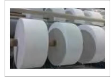
3- Cut off the edges on both sides, eventually become a non woven coiled material.
